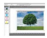
option you can generate CIP3 PPF Files up to Version. 2.0, related to the specifications of the CIP4 organization. With this CIP3 data, you can then make pre-adjustments of the ink keys of compatible printing presses.
